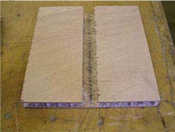
Another method of fixing shelves or bulkheads is by attaching a spline with epoxy then dado the core from the adjoining panel the depth of the spline, brush in thickened epoxy and slip the panel over the spline. (See
