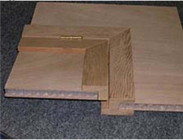
Counter tops and table tops, or shelf edges can be accomplished by cutting your edge molding to the desired shape and brushing in epoxy then bonding it to the panel. (See figure 16)
