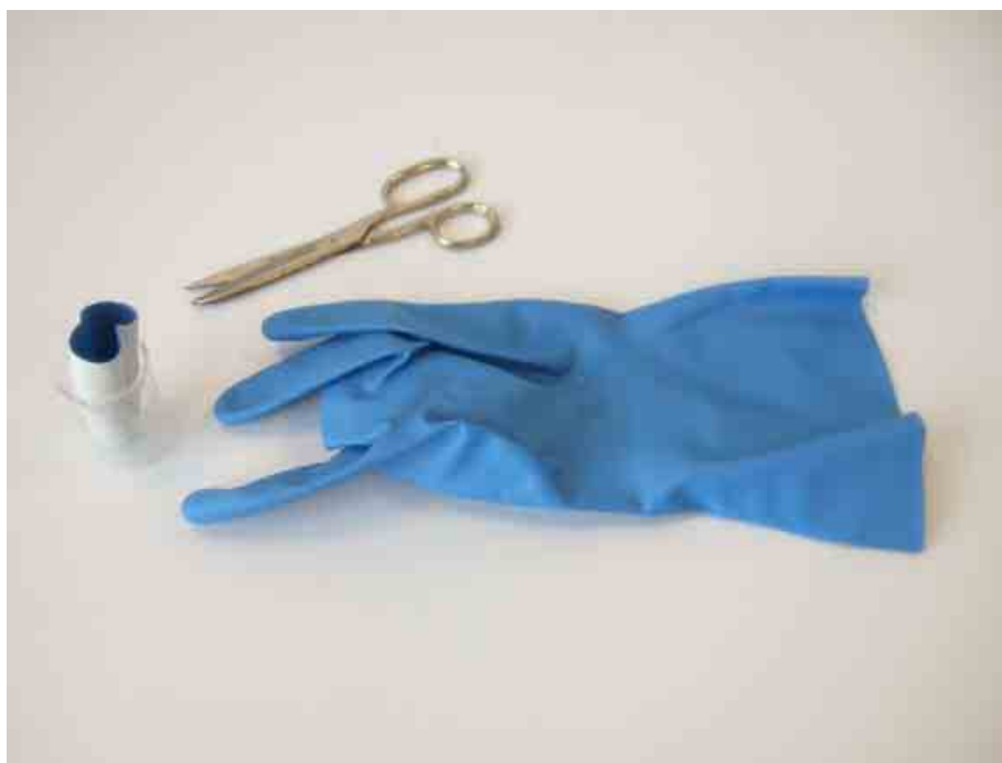
Figure 2.1 Experimental set up for 4-hour continuous contact screening test featuring: inside-out finger of glove placed upright in a beaker. The test liquid is pipetted carefully into the inside-out finger of the glove
