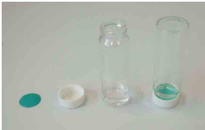
Figure 3.1 Experimental set up for the swelling tests featuring (left-to-right) glove material gasket; lid; bottle containing test liquid and assembled test
