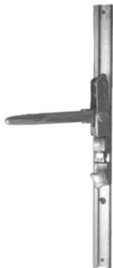
This all brass dinghy fitting consists of a spike on a gooseneck with tangs and thumb screw for adjustment. Supplied with 12" (300mm) of brass internal track, size ⅝" (16mm).
