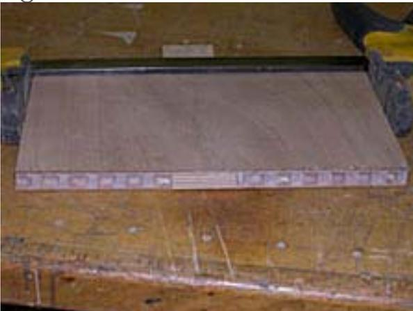
If a radius is required, kerf the panel at the starting point of the radius. Clamp the panel to a flat surface and raise the loose end until the kerf is closed. Measure the distance between the raised portion and the surface of the
