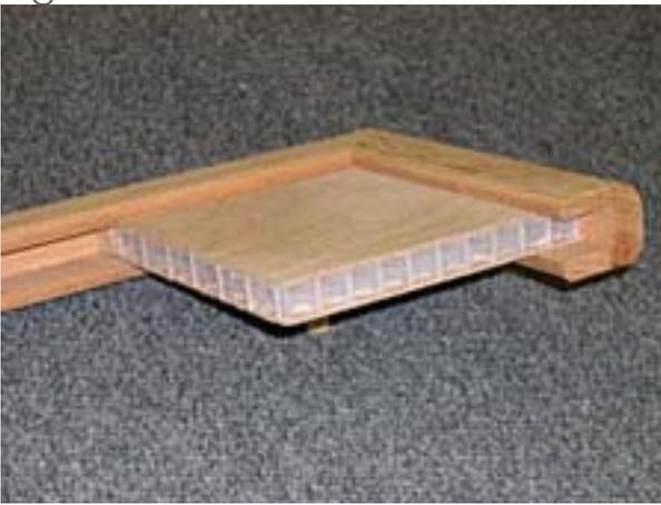
When using a cored panel, careful planning will eliminate problems encountered once the cabinet is assembled. There is very little extra time involved but the end result will be a very strong and lightweight cabinet.
