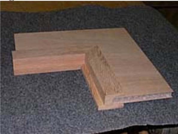
Cutting a dado into a solid frame, and gluing the Nida-Core panel into the dado can accomplish door frames. There is no special treatment to the panel. (See figure
